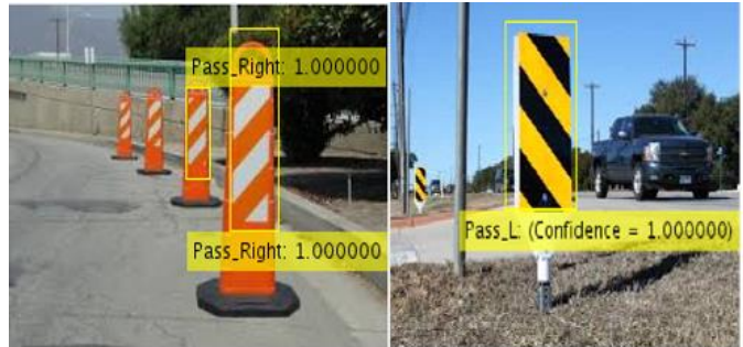
Figure 6: Labeled output image of different stripe pattern and color
